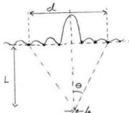
$$1. a) \frac{1}{2} kb \sin \theta = 3\pi \Rightarrow \frac{\pi}{\lambda} b \frac{d/2}{L} = 3\pi \Rightarrow b = \frac{6\lambda}{d} L = 0,13500 \text{ mm.}$$
